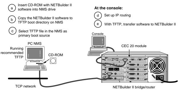
Figure 4-2 Installing NETBuilder II Software from CD-ROM on a PC NMS
